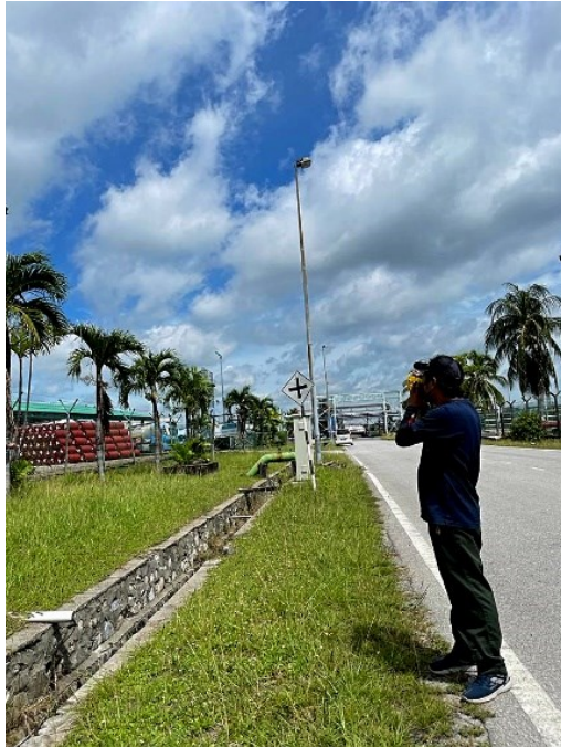
Figure 2.7 Height estimation using hypsometer
