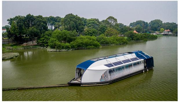
▲ Part-funded by Westports. Solar-powered Interceptor 002 can collect 10,000 kg of solid waste from Klang River
