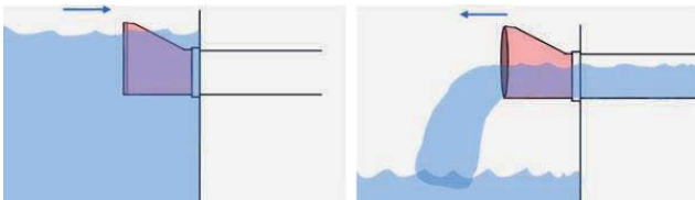
A duckbill check valve at the end of a pipe outfall in closed position (left, at high tide) and open position (right, at low tide, conveying stormwater runoff).
